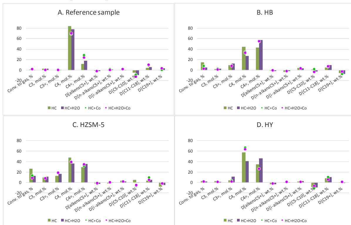
Fig. 1. The influence of the contact composition on the hydrocarbons mixture transformation
